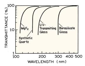
Figure 2.30. Typical transmittance of PMT window materials.
