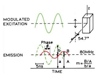
**Figure 4.2.** Phase-modulation or frequency-domain lifetime measurements. The ratios B/A and b/a represent the modulation of the emission and excitation, respectively.
