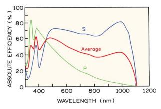
**Figure 2.14.** Grating efficiency for a 1800 line/mm halographic grating, optimized for the UV. The bold line is the average, and the other lines are for differently (S and P) polarized light, defined in Figure 2.39. Redrawn from [11].
