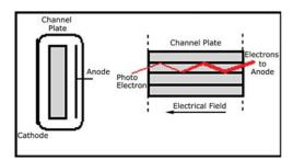
**Figure 4.24**. Photograph and schematic of an MCP PMT. The diameter of the housing is about 45 mm. Revised from [90–91].
