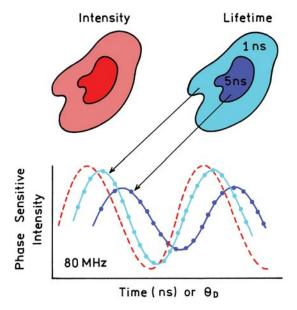
Figure 22.3. Schematic of lifetime imaging using phase-sensitive images.
