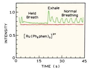
**Figure 19.10.** Luminescence intensity of an oxygen sensor with  $[Ru(Ph_2phen)_3]^{2+}$  as the probe, when exposed to breathing. Revised from [24].
