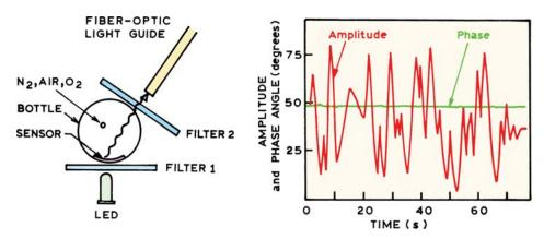
Figure 19.11. Phase-angle stability with intensity fluctuations measured with an oxygen-sensing device. The amplitude of the incident light was varied by waving fingers between the LED and the sensor. Revised from [33].
