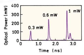
**Figure 4.11**. Pulsed picosecond laser diode emitting at 370 nm. The FWHM is less than 70 ps with a maximum repetition rate of 40 MHz. From [18].
