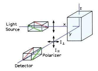
Figure 10.1. Schematic diagram for measurement of fluorescence anisotropies.
