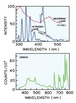
**Figure 4.21**. Spectral output of flashlamps. The output of the deuterium lamp is 100-fold less than of the nitrogen lamp. It is possible that emission below 600 nm for argon is due to impurities. Revised from [16] and [53].
