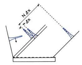
**Figure 4.28**. Path length difference across a monochromator grating. N is the total number of facets in the grating and  $\Delta x$  in the path length difference between adjacent reflections. From [126].
