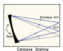
Figure 2.11. Monochromators based on a plane (top) or concave (bottom) grating. Revised from [7].
