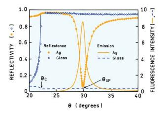
**Figure 26.4.** Reflectivity curves for a bare glass and silver-coated glass, both spin coated with a fluorophore in polyvinyl alcohol. The prism is LaSFN9 glass, 633 nm. Also shown is the fluorescence from the labeled PVA film on the glass and silver surfaces. Adapted from [11].
