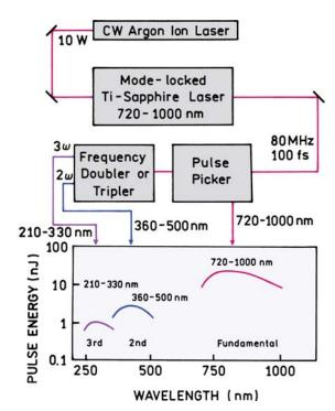
Figure 4.16. Mode-locked femtosecond Ti:sapphire laser.
