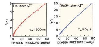
**Figure 19.9.** Stern-Volmer plots for oxygen quenching of  $[Ru(phen)_3]^{2+}$  and  $[Ru(Ph_2phen)_3]^{2+}$  in GE RTV 118 silicon. Phen is 1,10-phenanthroline; ph<sub>2</sub>phen is 4,7-diphenyl-1,10-phenanthroline. Revised from [24].
