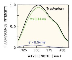
**Figure 17.6.** Spectral resolution of the short and long ns decay components of tryptophan. Similar results were reported in [5–6]. From [30].
