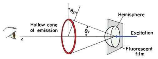
Figure 26.7. Surface plasmon-coupled cone of emission for fluorophores near a metallic film.
