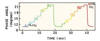
**Figure 19.22.** CO<sub>2</sub>-dependent phase angles of [Ru(dpp)<sub>3</sub>]<sup>2+</sup> in the sensor matrix containing Sudan III. The output of the LED was modulated at 20 kHz. Revised from [69].
