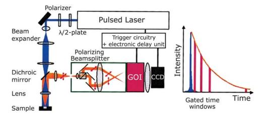
Figure 11.32. Instrument for correlation time imaging. Revised from [105].
