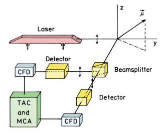
**Figure 24.45.** Measurement of photon antibunching and rotational diffusion by FCS. CFD, constant fraction discriminator. TAC, time-to-amplitude converter. MCA, multichannel analyses. Revised from [150].
