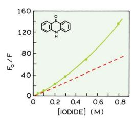
Figure 8.77. Iodide quenching of acridone. Data from [175].
