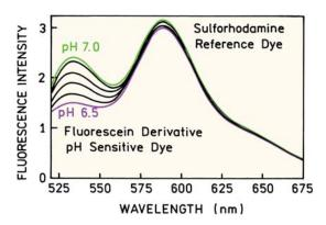
**Figure 19.64.** Emission spectra of a Pebble sensor, a polyacrylamide bead containing fluorescein as a pH-sensitive dye, and sulforhodamine as a pH-insensitive reference dye. Reprinted with permission from [238]. Copyright © 1999, American Chemical Society.
