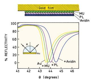
**Figure 26.3.** SPR reflectivity curves for a 47-nm gold film on BK-7 glass. Illumination was at 633 nm. The gold film was progressively coated with 11-mercaptoundecanoic acid (MU), followed by biotiny-lated poly-lysine (PL), and then avidin. Adapted from [7–9].
