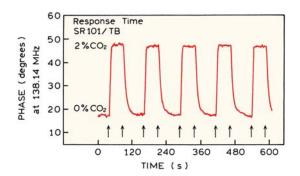
**Figure 19.82.** Response of an RET pCO<sub>2</sub> sensor employing SR 101 as donor and TB as acceptor to changes in the percentage of  $CO_2$  between 0 and 2%. The phase-angle measurements were made at a light modulation frequency of 138.14 MHz. From [65].
