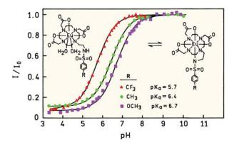
Figure 20.16. Lanthanide-based pH sensor. From [66].
