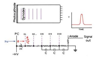
Figure 2.29. Schematic diagram of a photomultiplier tube and its dynode chain.
