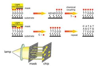
**Figure 21.63**. Light-directed synthesis of oligonucleotide arrays. From [189].
