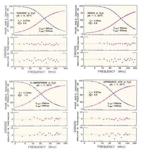
Figure II.9. Representative frequency-domain intensity decays. From [5].
