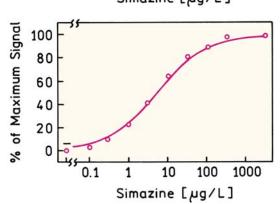
**Figure 19.73.** Competitive RET immunoassay for the herbicide simazine. Revised and reprinted with permission from [283]. Copyright © 2001, American Chemical Society.
