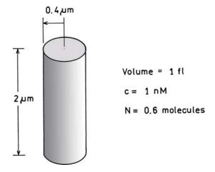
Figure 24.1. Typical volume in an FCS experiment.
