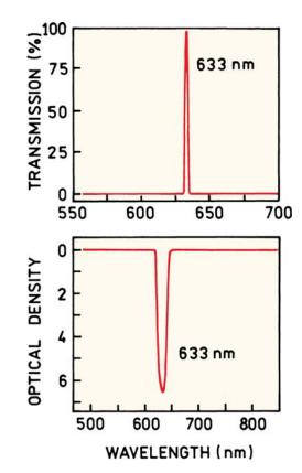
**Figure 2.20.** Laser line filter to transmit only the laser wavelength (top) and a notch filter to reject the laser wavelength. From [15].
