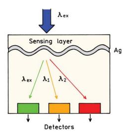
**Figure 26.17.** Fluorescence-sensing module based on grating-coupled plasmon emission.
