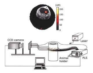
**Figure 19.68.** Schematic of an instrument for three-dimensional small animal imaging. PLS, programmable light switch. The image shows a sagittal section of a combined MRI and fluorescence image of a mouse injected with a cathepsin B-sensitive molecular beacon. From [258].
