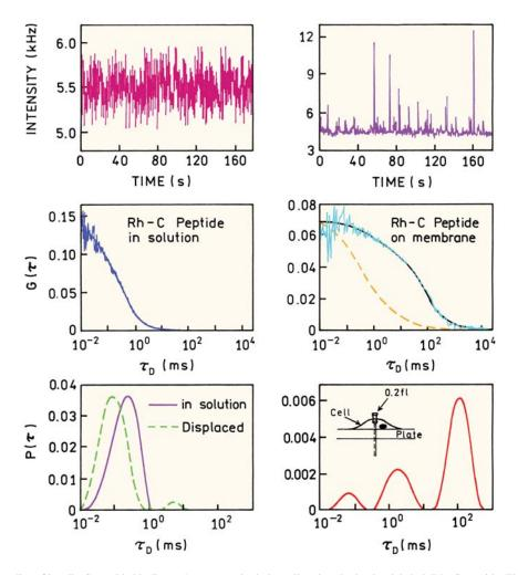
**Figure 24.22.** FCS studies of insulin C-peptide binding to human renal tubular cells using rhodamine-labeled (Rh) C-peptide. The dashed lines show  $G(\tau)$  and  $P(\tau)$  after addition of a 1000-fold excess of unlabeled C-peptide. Revised from [71].
