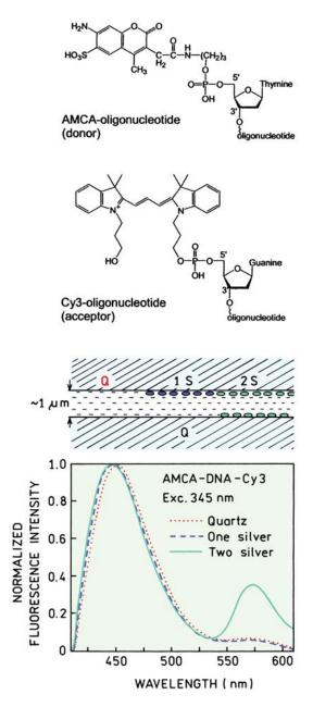
**Figure 25.31**. Effect of one or two SIFs on RET between AMCA and Cy3 bound to DNA. From [56].
