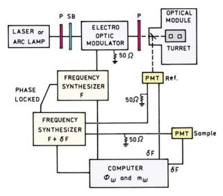
**Figure 5.7.** Schematic representation of the variable-frequency phase-modulation fluorometer. P, polarizer; SB, Soliel-Babinet compensator; F, frequency;  $\delta F$ , cross-correlation frequency; PMT, photomultiplier tube.
