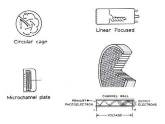
Figure 2.33. Types of PMT dynode chains. From [14].
