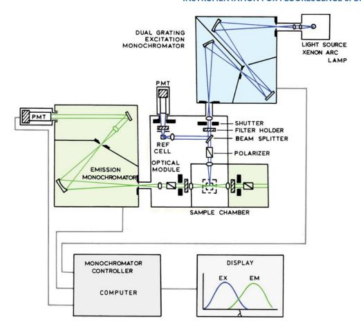
Figure 2.1. Schematic diagram of a spectrofluorometer [1].
