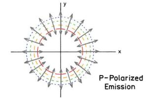
Figure 26.8. Color distribution and polarization expected for SPCE.
