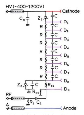
**Figure 5.10**. Dynode chain for an R928 photomultiplier tube used in a frequency-domain fluorometer. Revised from [1] and reprinted with permission from the Biophysical Society.
