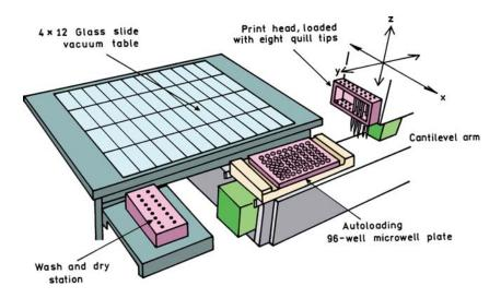
Figure 21.59. Apparatus for making spotted DNA microarrays. From [175].
