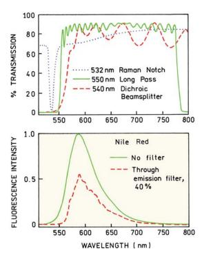
Figure 23.16. Emission filters and emission spectra of Nile Red in methanol. Revised from [16]. Revised and reprinted with permission from [16], Copyright © 2003, American Institute of Physics.
