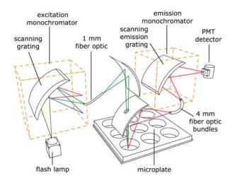
Figure 2.3. Optical path for a microplate reader [2].
