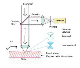
Figure 23.6. Principle of epifluorescence with confocal detection.
