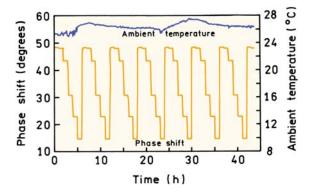
**Figure 19.13**. Lifetime-based sensing of oxygen using platinum (II) octaethylporphyrin ketone in a polymer membrane. The light modulation frequency is 3907 Hz. The gaseous oxygen concentrations were 0, 0.1, 5.1, 9.96, and 20.55%. Revised from [39].
