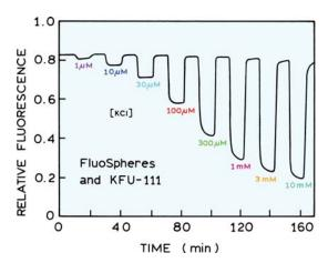
**Figure 19.28**. Response time, relative signal change, and reversibility of the potassium sensor in the presence of dye KFU 111 in the membrane; pH 5.82, excitation/emission wavelengths set to 560/605 nm. The sensor did not respond to potassium without KFU 11. Revised and reprinted with permission from [85]. Copyright © 1993, American Chemical Society.
