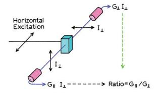
Figure 10.12. Schematic diagram for T-format measurements of fluorescence anisotropy.
