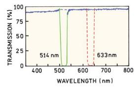
Figure 23.15. Transmission profiles of laser notch filters.
