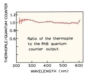
**Figure 2.42.** Comparison of the thermopile and the rhodamine B quantum counter as radiation detectors. Redrawn from [26].
