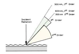
**Figure 2.16.** First- and second-order diffraction off a diffraction grating. The region where there is no overlap of the 1st- and 2nd-order diffraction is called the free spectral range.
