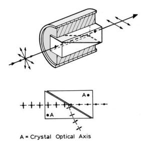
Figure 2.41. Glan-Thompson polarizer (top) and light paths (bottom).
