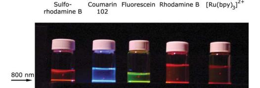
Figure 18.7. Simultaneous excitation of several fluorophores using the 800-nm output of a regeneratively amplified Ti:sapphire laser. The laser is incident near the bottom of the bottles. The upper lines are reflections off the surface. From [21].
