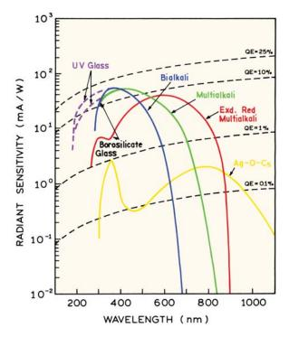
Figure 2.31. Spectral response curves of typical photocathodes. From [18].
