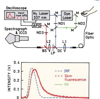
**Figure 4.34.** Time-resolved instrument using a high-speed oscilloscope for measuring of time-resolved decays of skin of human skin. Revised from [150].
