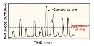
Figure 2.35. Photon-counting detection using a PMT. From [19].
