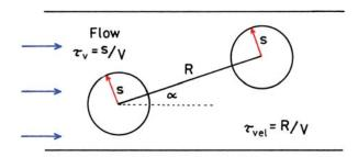
Figure 24.47. Flow velocity measurements using FCS.
