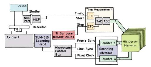
Figure 22.13. Schematic for FLIM using TCSPC. Revised from [40].
