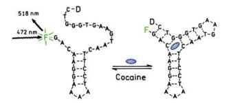
**Figure 21.40**. Structure of DNA aptamer that binds cocaine; F is fluorescein and D is dabcyl. Reprinted with permission from [126]. Copyright © 2001, American Chemical Society.
