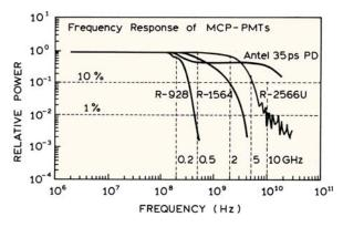
**Figure 5.24.** Measured frequency-response of several PMTs, and a fast photodiode (PD). Data from [107] and [108], and technical literature from Hamamatsu Inc.
