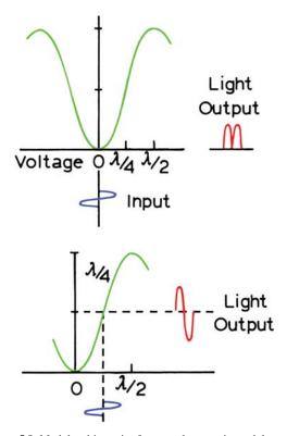
**Figure 5.9**. Modulated intensity from an electrooptic modulator. The upper drawing shows the modulated intensity without an electrical or optical bias, the lower drawing includes a  $\lambda/4$  bias.
