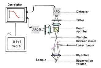
Figure 24.4. Typical instrumentation for FCS. Revised from [17].
