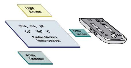
Figure 19.2. Fluorescence sensor for point-of-care testing.
