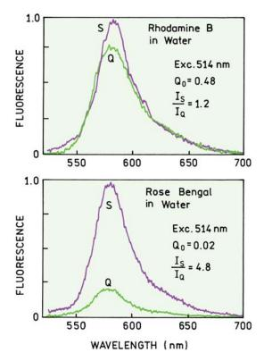
**Figure 25.16.** Emission spectra of rhodamine B (top) and rose bengal (bottom) between silver island films (S) or unsilvered quartz plates (Q). From [36].
