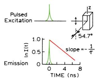
Figure 4.1. Pulse or time-domain lifetime measurements.
