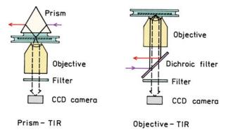
Figure 23.7. Optics for SMD imaging based on total internal reflection. Revised from [16].
