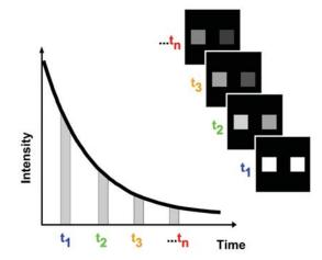
**Figure 22.10.** Schematic of FLIM using a gated-image intensifier. Reprinted with permission from [35].
