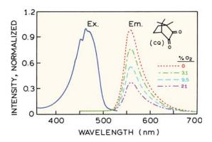
**Figure 19.79.** Normalized excitation and emission spectra of camphorquinone in poly(vinyl chloride) (PVC) illustrating the effect of oxygen concentration on phosphorescence intensity. Revised and reprinted from [308]. Copyright © 1994 with permission from Elsevier Science.
