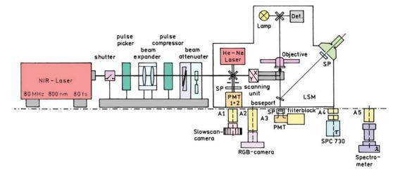
Figure 18.19. Schematic of a multiphoton microscope. Revised from [52].
