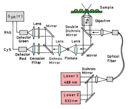
Figure 24.37. Instrumentation for dual-color FCS. Revised from [125].
