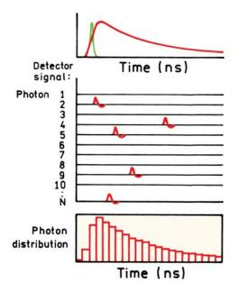
**Figure 4.7**. Principle of TCSPC. The pulses in the middle panel represent the output from a constant fraction discriminator (see Figure 4.22). Revised from [11].
