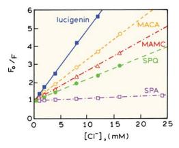
**Figure 19.17**. Stern-Volmer plots for chloride quenching of SPQ, SPA, lucigenin, MACA, and MAMC. See Table 19.1. Revised and reprinted with permission from [49]. Copyright © 1994, Academic Press Inc.
