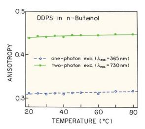
Figure 18.27. Steady-state anisotropies of DPPS. From [60].
