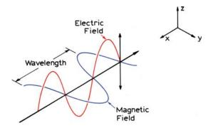
Figure 2.38. Vertically polarized light.
