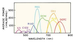
Figure 4.18. Output power of commonly used laser dyes.
