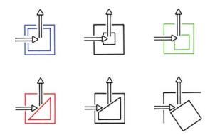
Figure 2.45. Various geometric arrangements for observation of fluorescence.
