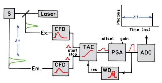
Figure 4.8. Electronic schematic for TCSPC. Revised from [14].
