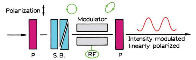
Figure 5.8. Optical arrangement for an electrooptic modulator. P, polarizer; SB, Soliel-Babinet compensator; RF, radio frequency signal. The SB compensator is replaced by an electrical DC voltage in some commercial FD instruments.
