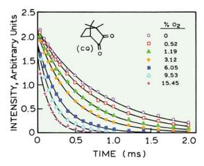
**Figure 19.80.** Phosphorescence lifetime measurements for camphorquinone in poly(methyl methacrylate) (PMMA), illustrating the influence of oxygen concentration on the triplet decay. The polymeric supports are different in Figures 19.79 and 19.80. Revised and reprinted from [308]. Copyright © 1994 with permission from Elsevier Science.
