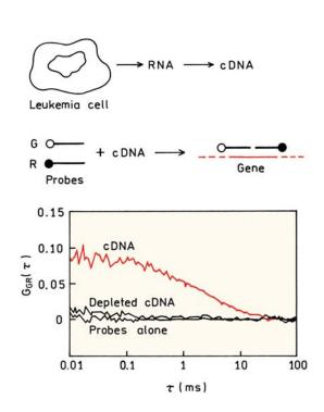
**Figure 24.42.** Detection of gene expression using dual-color FCCS. Revised from [137].
