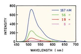
**Figure 2.37.** CCD spectrofluorometer and emission spectra of fluorescein. The light source for the fluorescein spectra was a 450 nm blue LED. From [25]. Image courtesy of Ocean Optics Inc.
