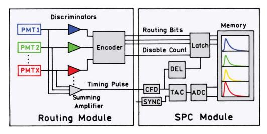
Figure 4.29. Electronic schematic for TCSPC with multiple detectors. Revised from [134].
