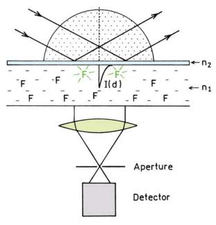
Figure 24.33. Experimental configuration for FCS using total internal reflection.
