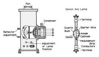
**Figure 2.7**. Xenon air lamp and a typical lamp housing. Revised from [5]. Courtesy of Newport Corp.
