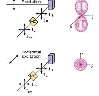
**Figure 10.11.** Schematic diagram for L-format measurements of fluorescence anisotropy. MC, monochromators. The shapes on the right are the excited-state distributions.
