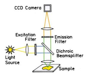
Figure 2.23. Filter geometry used for epifluorescence microscopy.
