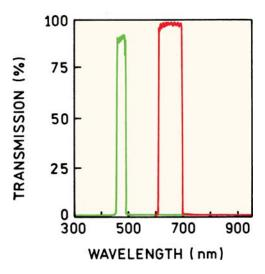
**Figure 2.21.** Interference filter to transmit selected wavelengths. From [15].
