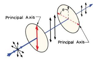
**Figure 2.40**. Transmission of light through polarizers. The incident beam is unpolarized. Only vertically polarized light passes through the first polarizer. Transmission through the second polarizer is proportional to  $\cos^2 \theta$ .
