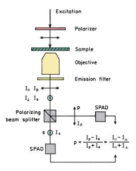
Figure 23.35. Typical configuration for single-molecule polarization measurements.
