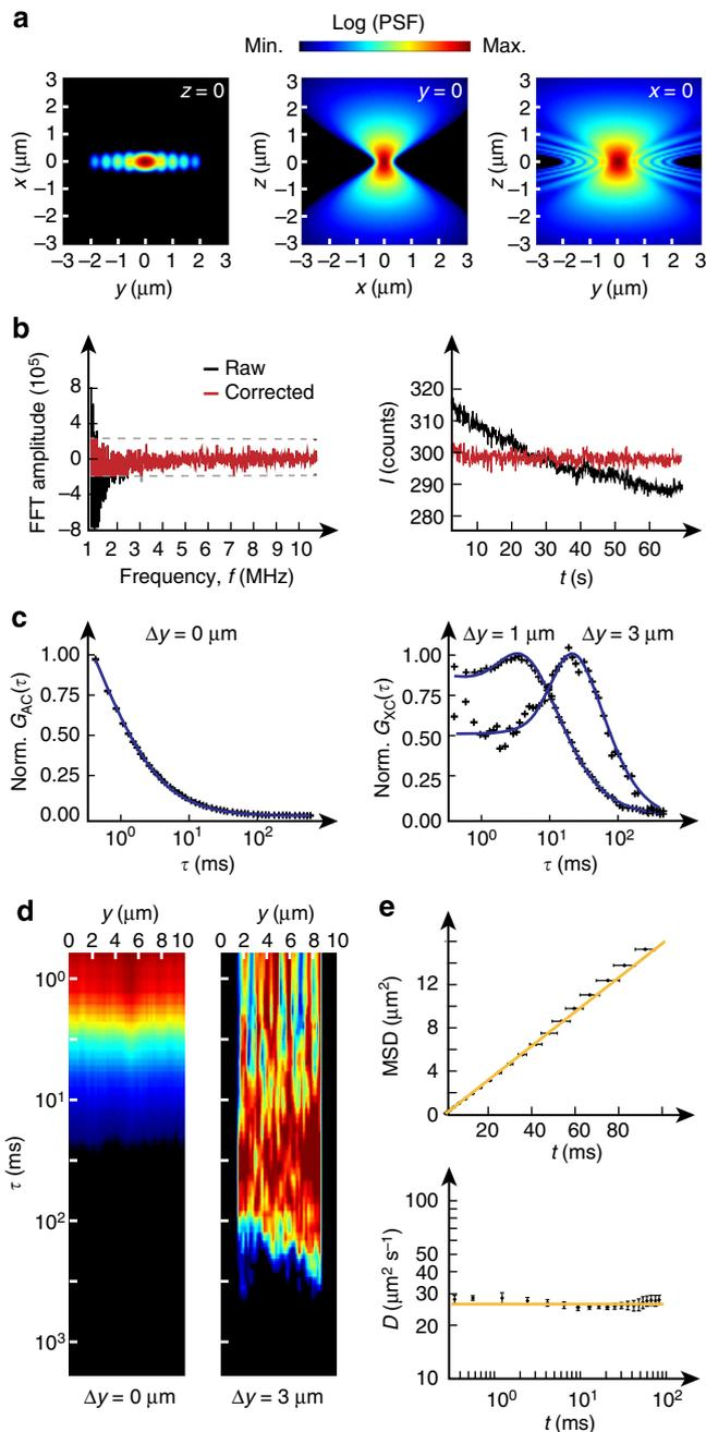
**Figure 2 | Instrument characterization, signal processing and validation of the data analysis pipeline.** (a) Approximation of the PSF of the line-confocal microscope as used for subsequent correlation analysis.
