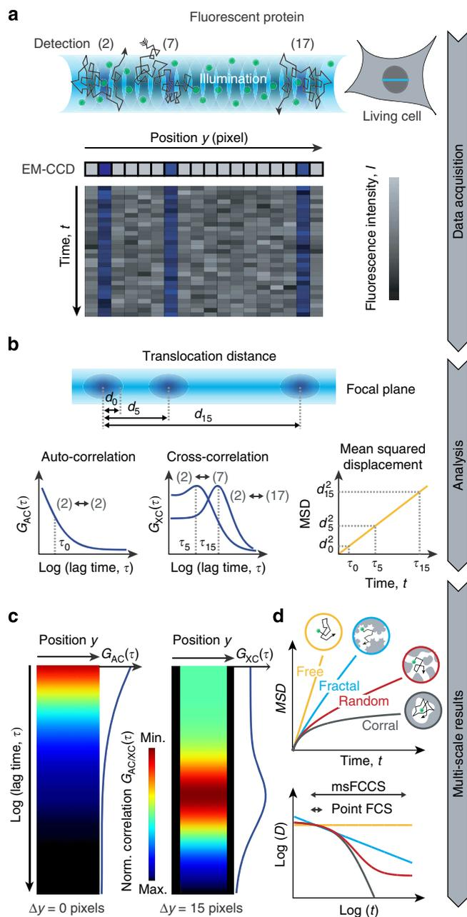
**Figure 1 | Parallelized acquisition of fluorescence signals for msFCCS**
