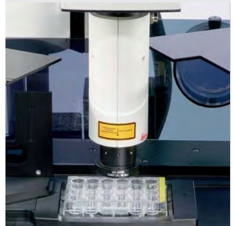
Adjusting of magnification by motorized zoom
