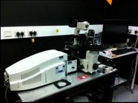
Scian/Leo-Lab: Perkin Elmer Spinning Disk with laser ablation
