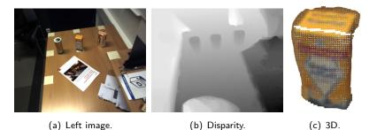
Figure : A robotics related disparity example. Based on the 3D 'image', the system detects the object and the decides upon how it can be manipulated etc.
