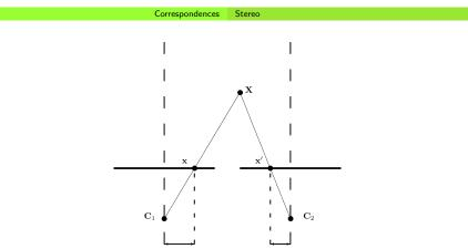
Figure :  $C_1$  and  $C_2$  are the camera centres of the respective cameras. **X** is the point of interest in 3D world coordinates, while **x** and **x'** are the images of the same on the respective camera planes. Disparity is d = x - x'.
