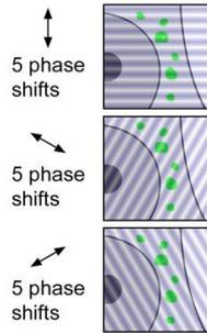
Interference of exciting light with sample structure (*Moiré effect*)
