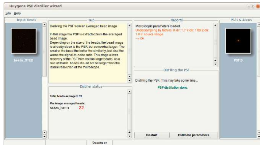
Figure 10.2: Estimating the STED microscopic parameters of a beads image automatically with the Huygens PSF distiller.
