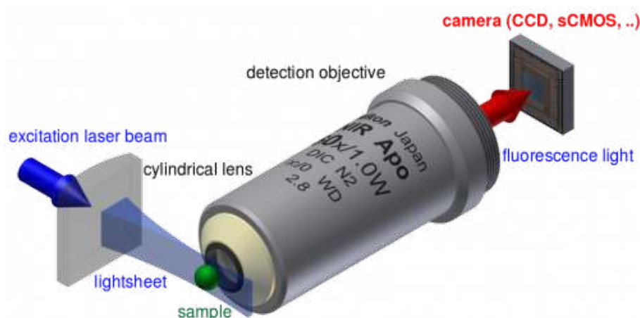
Figure 12.1: Principle of Light sheet fluorescence microscopy. The excitation light is shaped by a cylindrical lens in order to illuminate a thin plane of the sample. The objective is oriented perpendicular to the illumination plane to capture an image of a thin section of the sample
