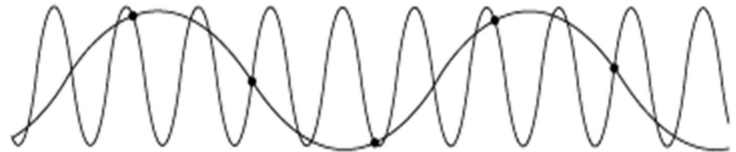
Aliased Signal Due to Undersampling
